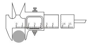
The quantity (M-V) is called  $\ensuremath{\textit{Vernier Constant}}\xspace (VC)$  or  $\ensuremath{\textit{Least Count}}\xspace (LC)$  of the vernier callipers.
