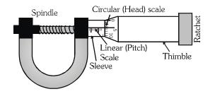
L.C. =  $\frac{\text{Pitch}}{\text{Total no. of divisions on the circular scale}}$  where pitch is defined as the distance moved by the screw head when the circular scale is given one complete rotation. i.e.
