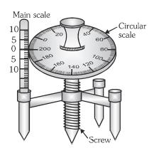
Radius of curvature =  $\frac{\ell^2}{6h} + \frac{h}{2}$ where  $\ell = \frac{\ell_1 + \ell_2 + \ell_3}{3}$ h= difference of readings taken on curved surface & that on flat surface.
